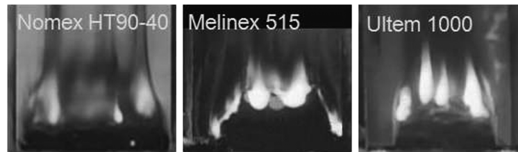
Fig. 5 Front-view pictures of 1 g upward flame spread at the ULOI (WSTF modified test 1 with hot-wire ignition). Samples are 5 cm wide in each image.
